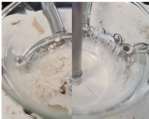
Comparison of the dispersions: on the left zinc oxide plus C_{12-15} alkyl benzoate only; on the right zinc oxide plus C_{12-15} alkyl benzoate with 5% of Olivem® 2090 (anchor stirrer at 450rpm for 10mins)
